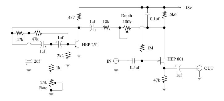
This tremolo circuit is not a "plug and play" ready guitar effect, however it could be converted to one with relative ease. It just needs some buffering on the input and ouput and perhaps some bypass switching.
